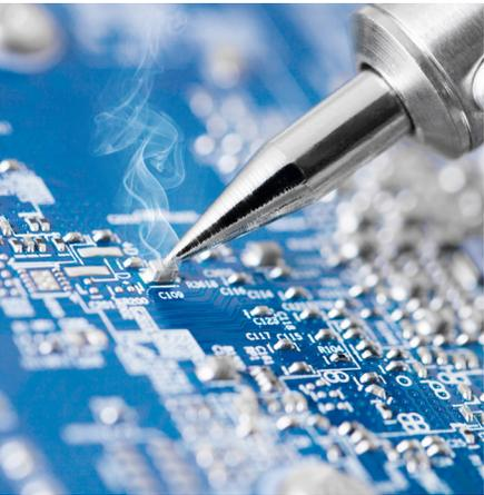
using copper salts and other plating chemicals. A solder mask (made of acrylic, polyurethane, or epoxy in combination with hardening agents and photoinitiators) is applied to insulate the copper and protect it from coming into contact with other materials. The solder mask is what gives PCBs their distinctive green color. Multiple layers can be constructed with epoxy laminate separating the layers.
